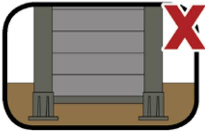
Please don't bury the bottom of the fence. A minimum gap of 30mm must be allowed for drainage at the bottom of each fence panel. Gravel can be used to hide the gap.
