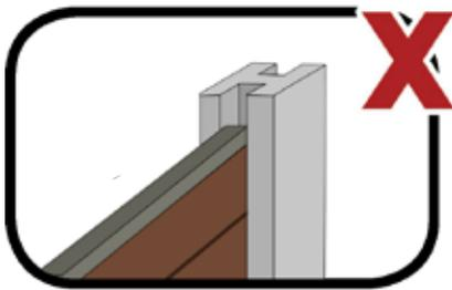
Our wall mounting post / insert (**72Pi18G**) must be used when installing our fencing into pre-existing concrete posts, buildings, wood posts or brick walls.
