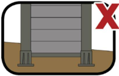
Never use Rinato Composite fencing as a gravel board or a structural product. Always bolt the bases to firm foundations. Do not bury them into the ground.
