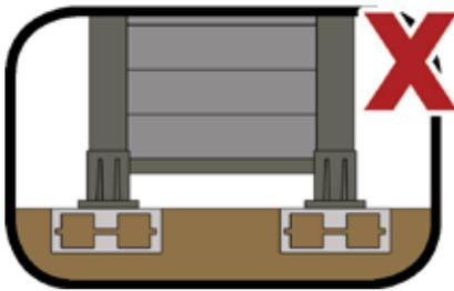
Do not fix posts to hollow bases such as breeze blocks.
