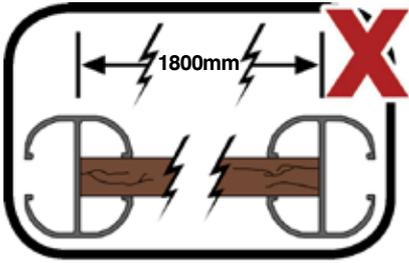
Always leave sufficient gaps at both ends of composite fence panels to allow for expansion otherwise you risk damaging the fence as a whole.
