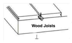
1. Place first piece of the decking at the edge perpendicular to the wood joist. Notch the decking to accommodate for the 100 x 100mm Post.
